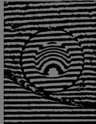
**Figure 4.11** (a) The principle of the Mach–Zehnder interferometer. (b) The interference fringe pattern obtained with an interference microscope from a graded index fiber
